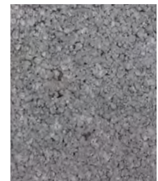
Porous concrete reduces the quantity of stormwater runoff.
