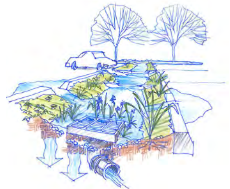
Bioswales are landscape strips with plants that convey and slow the speed of surface stormwater runoff, allowing water to infiltrate back into the ground.
