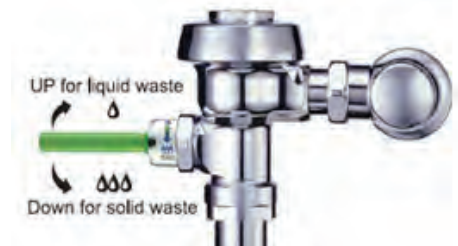
Sloan Dual Flush Handle Diagram http://greenasathistle.files.wordpress.com/2008/02/dual.jpg
